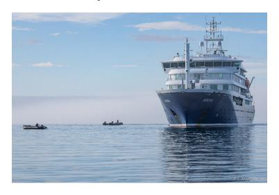
Hondius was built in 2019 in Split, Croatia. She is 107.6m long, 17.6m wide, and has a maximum draught of 5.3m. With an ice class of PC6, a top speed 15 knots, and three diesel generators, she sails on low sulfur marine gas oil and has a capacity of 176 passengers in 83 cabins. This comfortable, structurally advanced vessel is built from the ground up for polar adventure.
